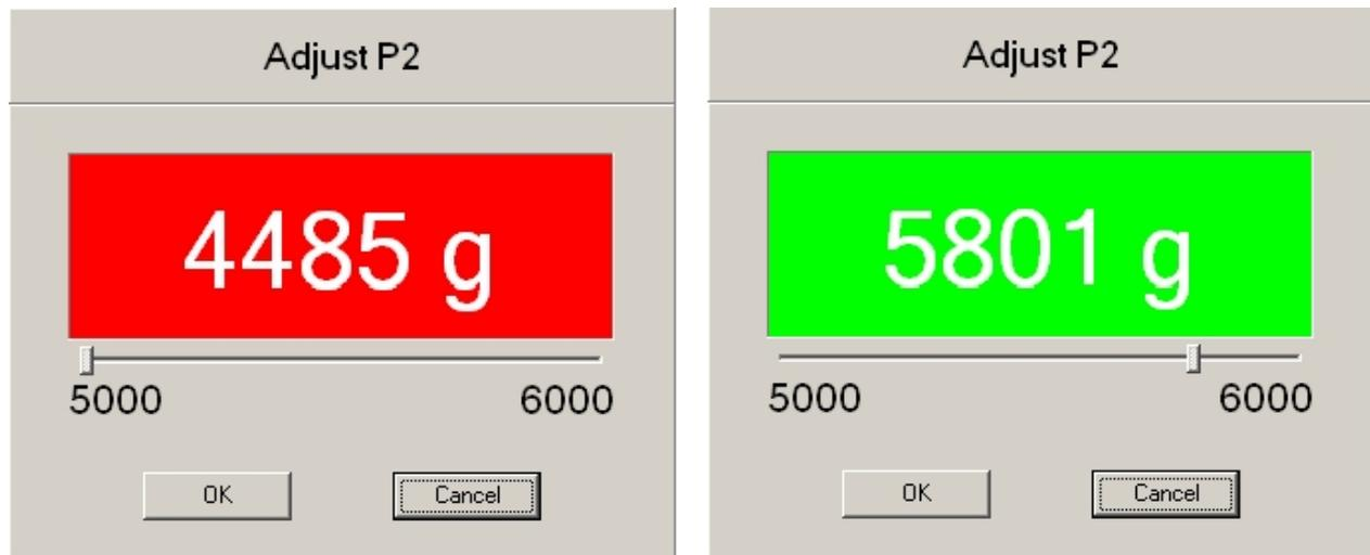
If the OK button is pressed, the actual value is checked on the valid range and determines whether the command passes or fails
